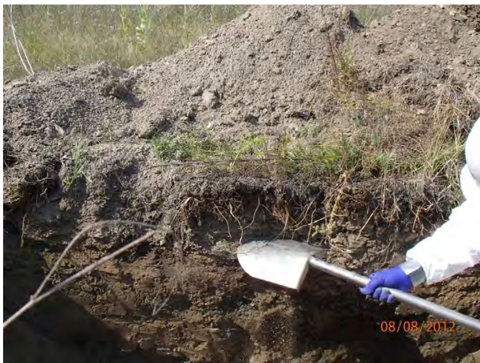
Photo 1. Excavation on west side of Rainey Creek showing an approximately 10-inch layer of dredge spoils overlying alluvial sediments.
