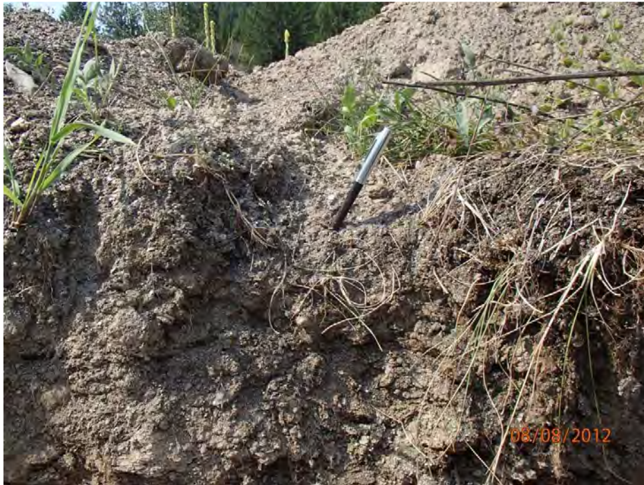
Photo 2. Close-up photo of dredge spoil materials showing coarse sand grain size and characteristic color.
