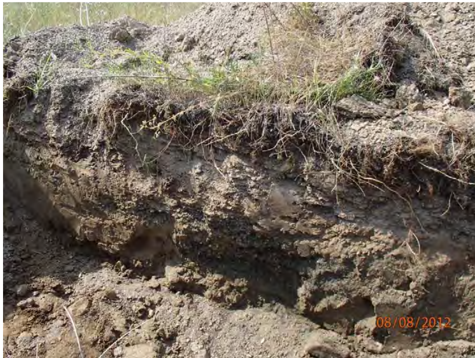
Photo 3. Bedding present in alluvial sediments underlying dredge spoils.
